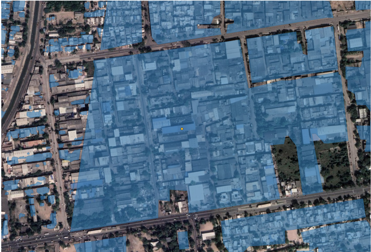
Figure 5: Example of the unwanted aggregation of multiple buildings to one LoD1-building-object within the city of Ahmedabad
